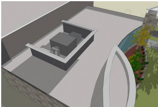
Provide architectural screening around roof-mounted mechanical equipment to minimize the visual impact from the street.
