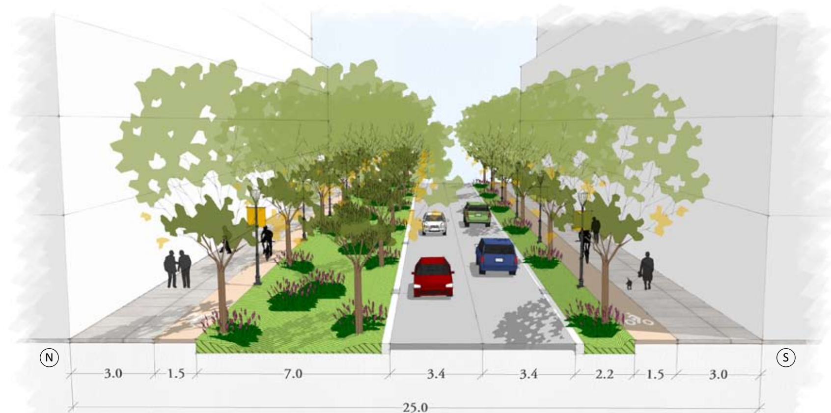
Mid-block City Centre Drive
