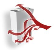
When wind hits the windward face of a tall building, the building tends to deflect the wind downwards, causing accelerated wind speeds at pedestrian level and around the windward corners of the building.
