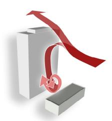
When the leeward face of a low building faces the windward face of a tall building, it causes an increase in the downward flow of wind on the windward face of the tall building.
