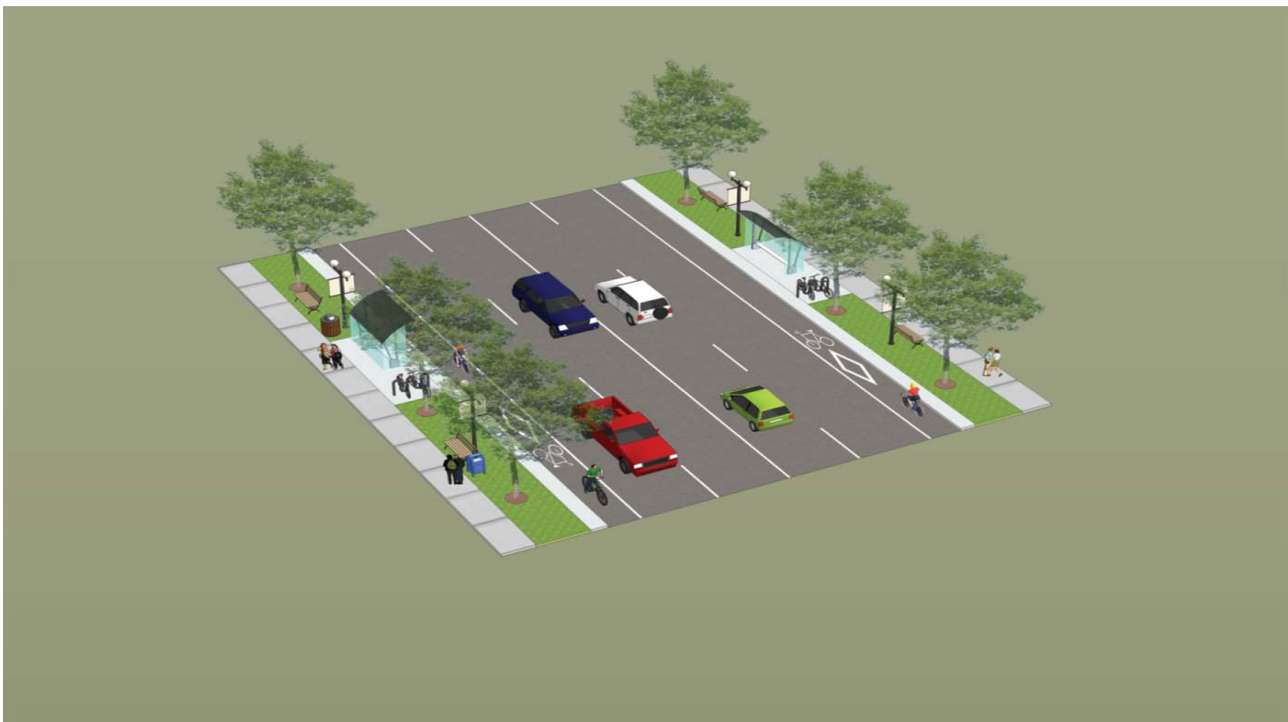
Figure 8-3: The ability to create multi-modal roadways will be influenced by right-of-way widths. Wider rights-of-way will allow for dedicated space for different transportation modes, however, where rights-of-way are narrower transportation modes will need to share space.
