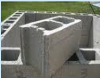
Figure B102 — Prohibited to be exposed: Concrete Block
