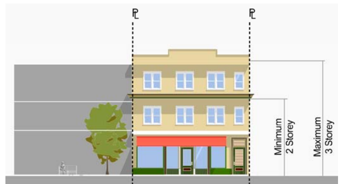
Figure 3-16 A minimum of 2 storeys and a maximum of 3 storeys is required for buildings fronting onto Lakeshore Road West in the north side of the Village Core. Also in other locations, the maximum is 4 storeys.
